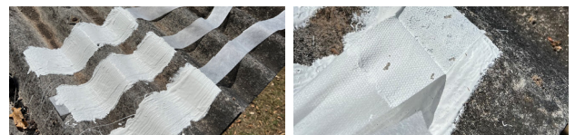
Adhesion test on aged asbestos roof
